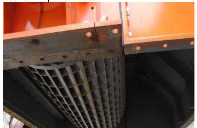
**Underside of the turbine showing the rotor blades which are driven by the water rushing down the penstock pipe**
