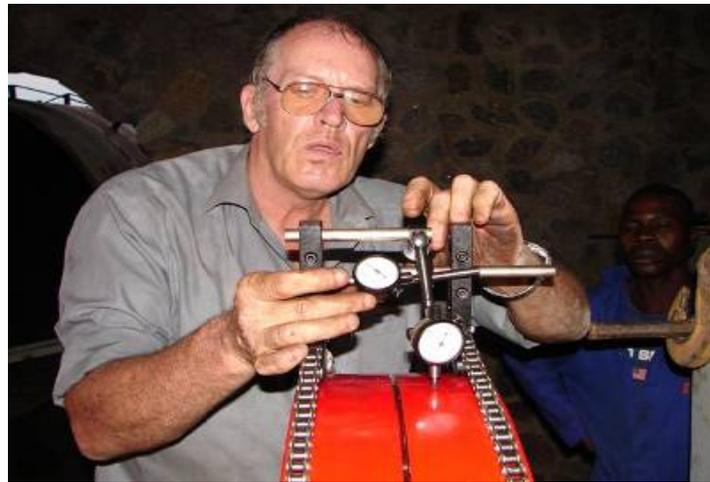
Alignment of the shaft and couplings from the Turbine and Gearbox
